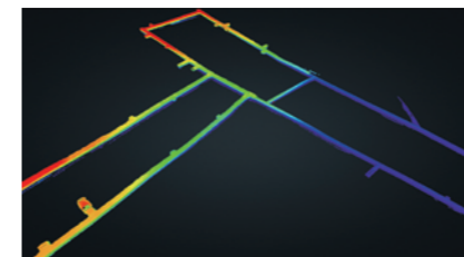
Mine Roadway Point Clouds
