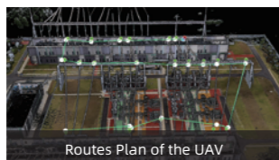
Point Clouds of Exchange Power Station
